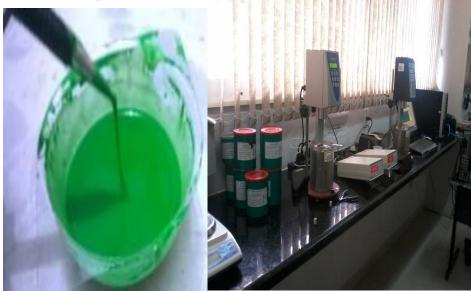
Soon the rheological study qualify the folder. Since, according to Souza et al (2011) it is possible to identify the characteristics of a given fluid. A fluid is as a substance that continually deforms when it's submitted a constant effort, no matter how small is this effort. Of all the properties of the fluid, the viscosity requires greater attention in the study of the flow of a fluid (Lopes, 2010).
